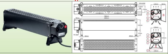
A: Floor mounting version (feet assembled under the frame); B: Wall mounting version (feet assembled on the side); 1: Waterproof knob, for mechanical or electronic thermostat; 2: Waterproof 2 poles on-off switch; 3: Waterpoof Led light; 4: Customisable stainless-steel identification label; 5: Rubber feet
